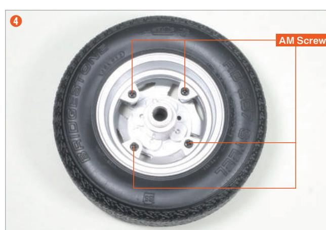
While holding both rims to prevent them from shifting, secure the four points with **AM Screws**.
