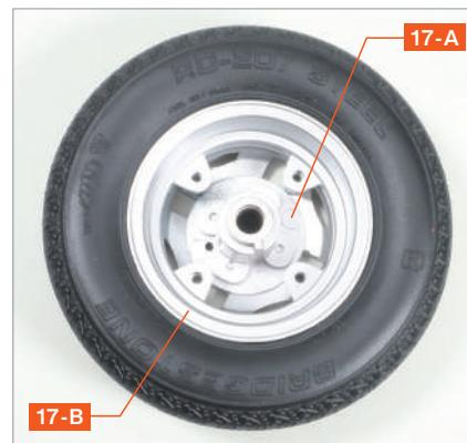
While holding **17-A** to prevent it from coming off, turn it over and align the recesses on the underside of **Inner Rim 17-B** with the protrusions of the screw holes on **17-A**, then fit it in.
