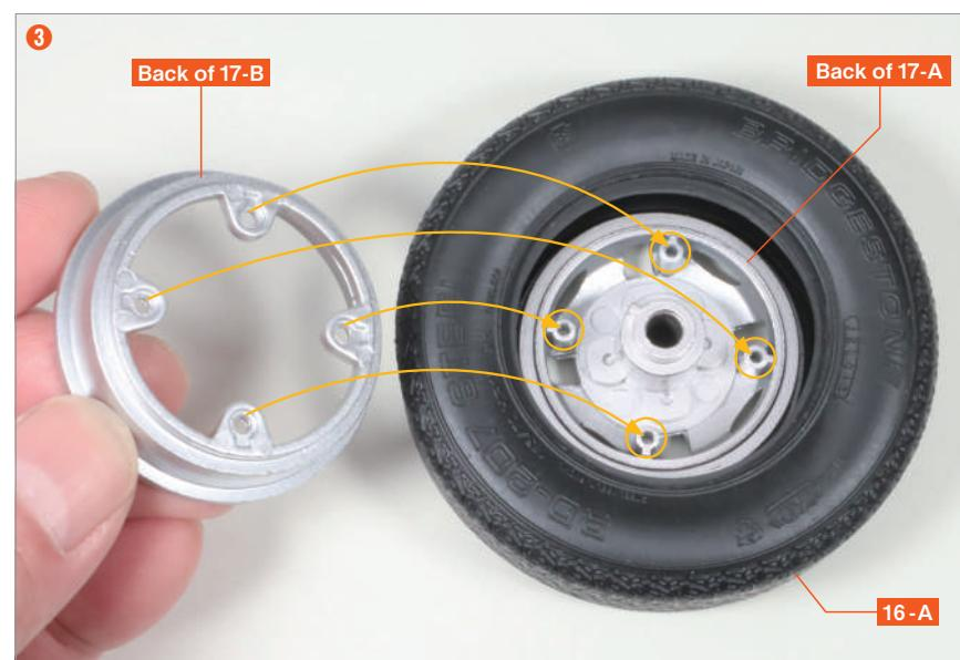
Precisely align the screw holes of **17-B** and **17-A**.
